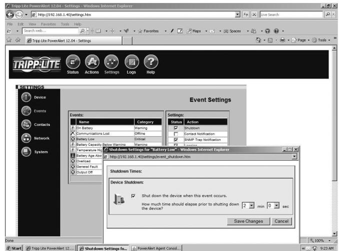
Figure 3-12: “Battery Low” Event Shutdown Settings
