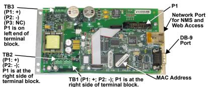
**DHCP**: The card ships with DHCP service enabled. The MAC address is printed on a sticker affixed to the top of the card.
